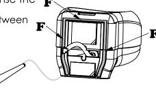
Solution Verify that the tube (c) is in the upper position and that the Dropper (5) is attached. Insert tube (c) into the hole (A) and press the dispenser into place based on the mark (D)
