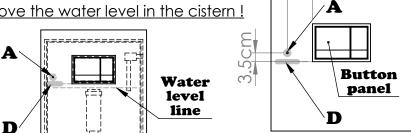
2 Drill a 7 millimeter hole (A) without vibration, Make sure that the hole is completely clean
